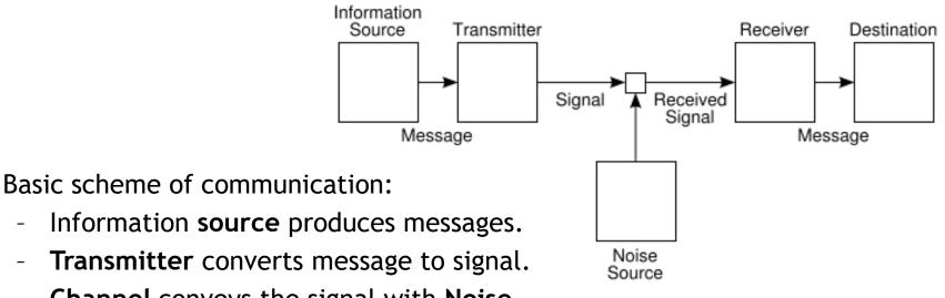
**Channel** conveys the signal with **Noise**. \_
