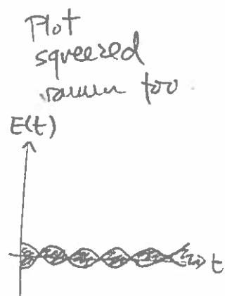
Key: Squeezing depends on the squeezing angle and is phase (time) dependent!
