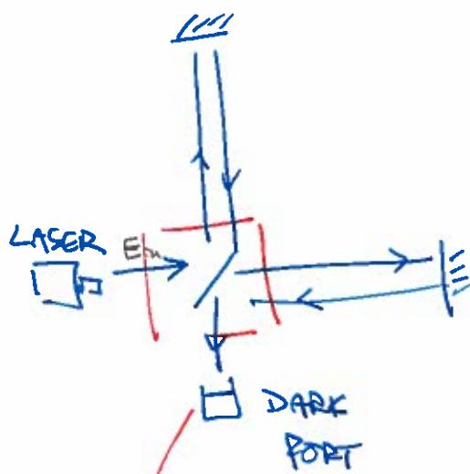
Usually, we ~~don't~~ think of the dark port simply as a readout port, where we do not inject any signal from the DP to the beamsplitter.
