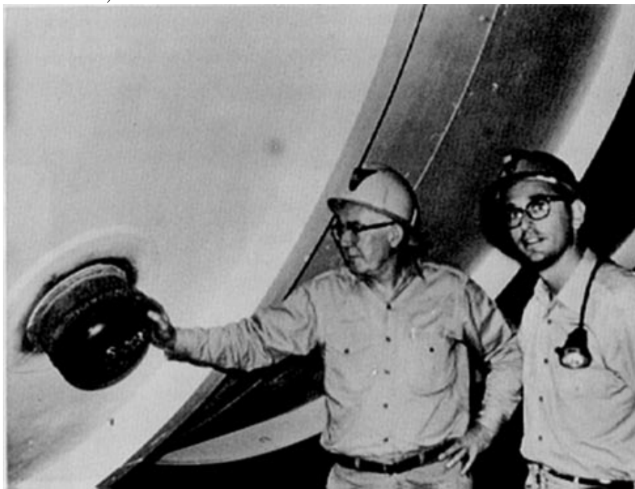
Ray Davis shows John Bahcall the tank containing 100,000 gallons of perchloroethylene. The picture was taken in the Homestake mine shortly before the experiment began operating.
